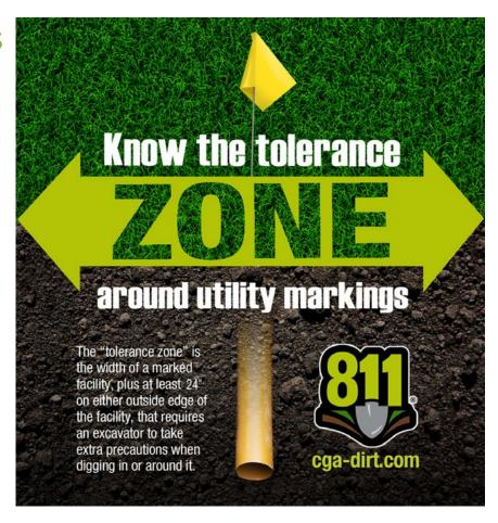
which alerts utility companies of the intent to dig. Professional locators are then dispatched to mark underground line locations with paint or flags. These marked lines show you where it is — and isn't — safe to break ground. Once your lines have been marked, make sure to dig carefully around the marks, not on top of them.
